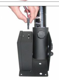
Plug in the electric cannon connector in the right way into the connector on top of the Power Shot.
